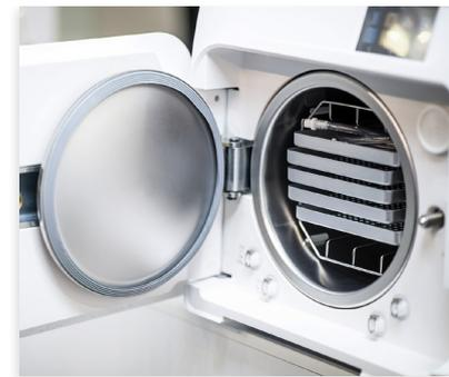
1. Place one test pack in the front of the chamber near the door, along with a normal load.
